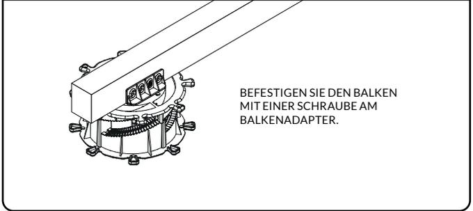
BEFESTIGEN SIE DEN BALKEN MIT EINER SCHRAUBE AM BALKENADAPTER.
