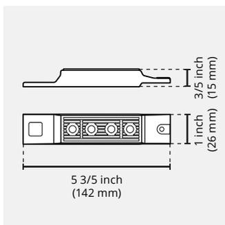
**Hidden deck fastener DECK-DRY** - clip with screws included, plank width 5 3/7 - 5 5/7 inch (138 - 145 mm) (20 pcs/sqm)
