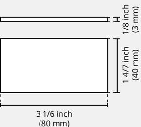
Rubber deck joist pads (3 1/6 × 1 4/7, 5/16 inch)
